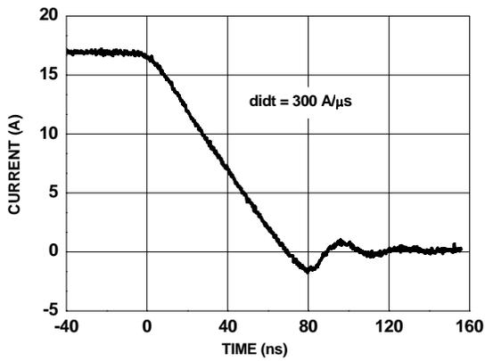
Figure 27. FDMS3669S SyncFET™ body diode reverse recovery characteristic
